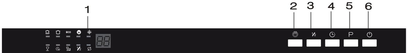
1. Display screen and lamp: to show the error code delay time etc.
