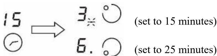
2. Once the countdown timer expires, the corresponding zone will switch off. Then it will show the new min. timer and the dot of corresponding zone will flash.
